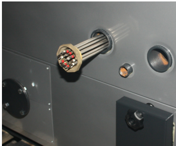
1. Installation of the resistance
