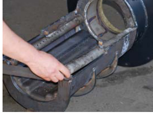
Removing air pipes
