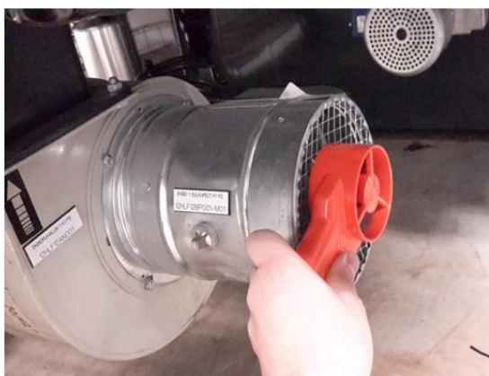
Figure 15. Air quantity measurement from the suction opening.
