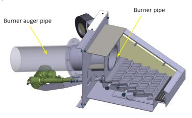
A drive motor and reduction gear are installed at the end of the burner auger. The permitted positions of the gear can be found at the end of the operating instructions. The picture shows wood chip-burning equipment.
